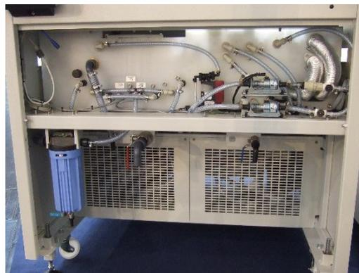
Easy access to all major components including pumps and motors via quick release and removable covers
